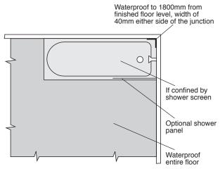
For timber floors including particleboard, plywood and other flooring materials apply Undertile Butynol® waterproofing membrane to entire floor
